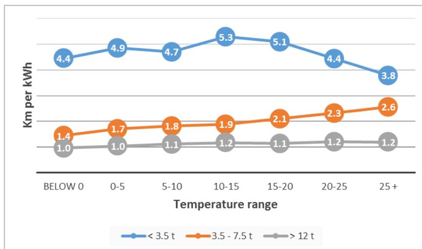
**Figure 7: Km per kWh depending on temperature range and weight groups**
