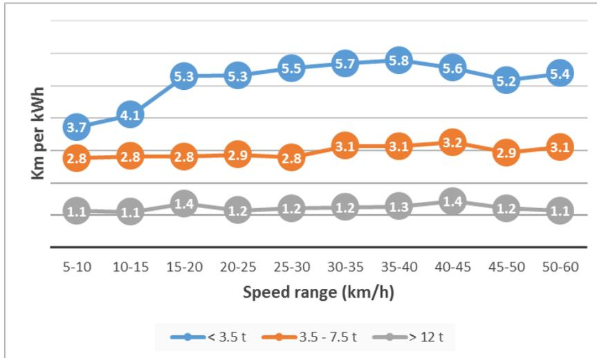
Figure 11: Km per kWh depending on average speed for weight groups
