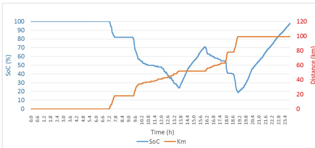
**Figure 4: Example of SoC and distance driven for a 24-hour period**
