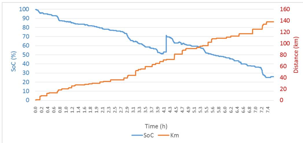
**Figure 5: Example of SoC and distance driven for a working day**
