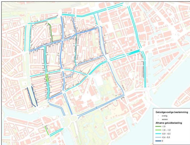
Figure II Noise reduction levels along 50 km/h roads
