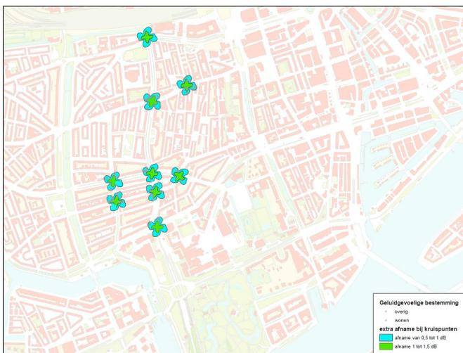
Figure III Additional noise reduction levels at and around intersections
